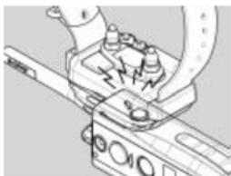
3. Place the red dot on the back of the transmitter against the red dot on the Black or Orange collar/receiver. Hold the two red dots together for several seconds, until the green LED on the receiver/collar starts to blink rapidly, and then separate the two red dots.
